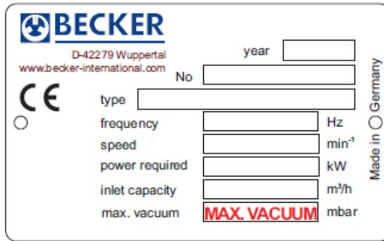
On every pump there will be the **pump nameplate**. It will state: the year the pump was manufactured, the serial number of the pump, the type of pump, frequency, rpm, kW (motor HP), volumetric flow inlet capacity, and the max vacuum. The data sheet will also provide this information.
