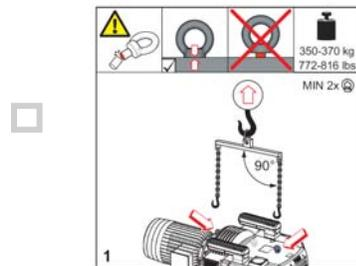
Make sure the eyebolts are fully screwed in. The position of the eyebolts fit to the center of gravity of a pump including the drive motor. If a pump without motor is to be lifted, attach another belt/rope at a suitable point.
