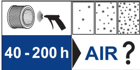
Filter/elements should be checked between 40-200 hours. The elements should be blown with compressed air from the inside out. Blast air should be felt coming through the filter/element. The element needs to be replaced if dirty or clogged. **Use only Becker Genuine filters to maintain warranty protection.**
