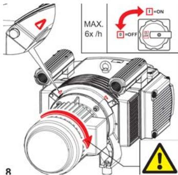
Locate the arrows that indicate correct rotation of motor/fan after electrical hook-up. Do **not reverse rotation** of the pump, this will spin the vanes backwards incorrectly and possibly break or chip vanes. **Bump** the drive motor and watch the fan wheel to determine the direction.
