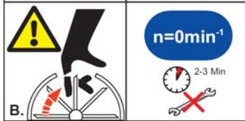
Caution: rotating unit. Do not work on the pump/motor until it is idle with no rotation. This may take up to 3 minutes. Follow proper lockout/tag-out procedures.
