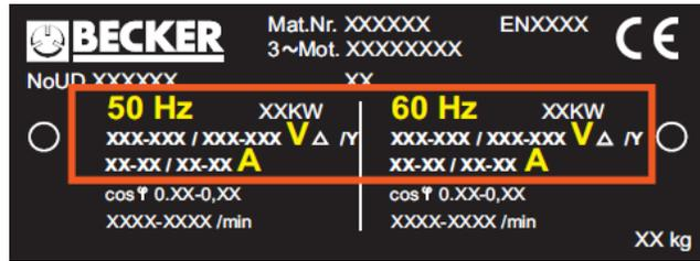
On every motor there will be the **motor nameplate**. It will state the motor electrical information with kW, Hz, voltage, amps, speed, with the wiring diagram on the motor nameplate or inside the motor box, IP rating, UL/CSA recognition, and operating mode (S1).
