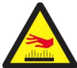
The vacuum pump will become **very hot** during operation. This is normal. Care should be taken to let the unit cool down before maintenance. **(High temps: 175+ degrees F (79+ degrees C)**
