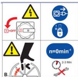
Caution: rotating unit. Do not work on the pump/motor until it is idle with no rotation. This may take up to 3 minutes. Follow proper lockout/tag-out procedures.
